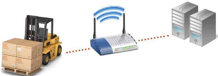
*With a DAP tablet mounted on a forklift, operators can seamlessly roam between access points, giving them freedom to move throughout the entire warehouse without losing wireless connectivity.*
