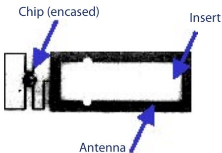
**Figure 3: Finished Tag – Pallet Tag**
