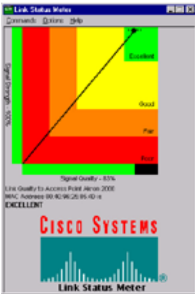
Figure 3. Site survey tools included with Cisco Aironet Client Utility assist in the correct placement of access points.
