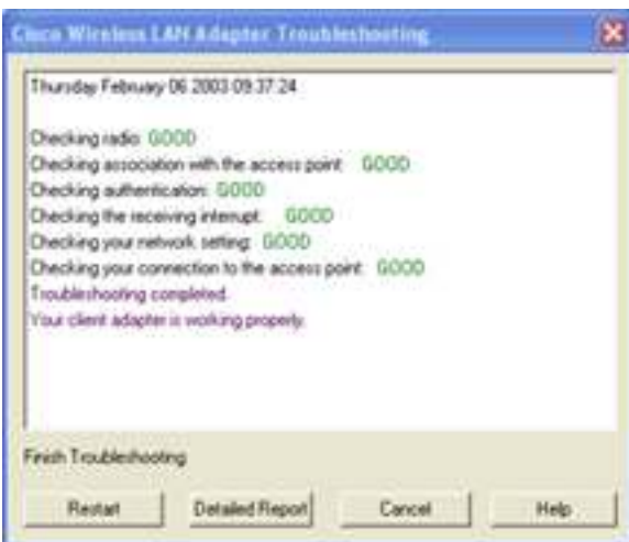
Figure 4. Troubleshooting Facility gives step-by-step details on the process of connecting to an access point.
